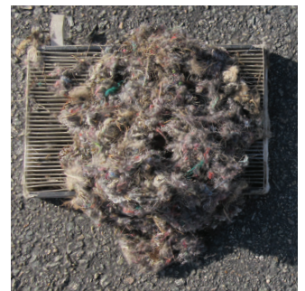
Cabin air filter that has not been replaced within the recommended 12,000 – 15,000 miles
